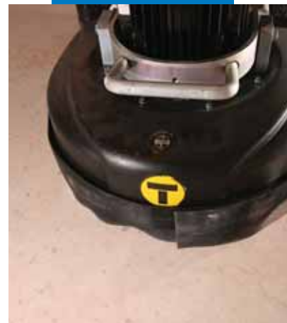
Dry-polishing process of Ultratop/Dynastone Color mix after hardening
