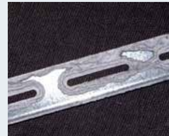
Grid component that has been affected by white rust.
