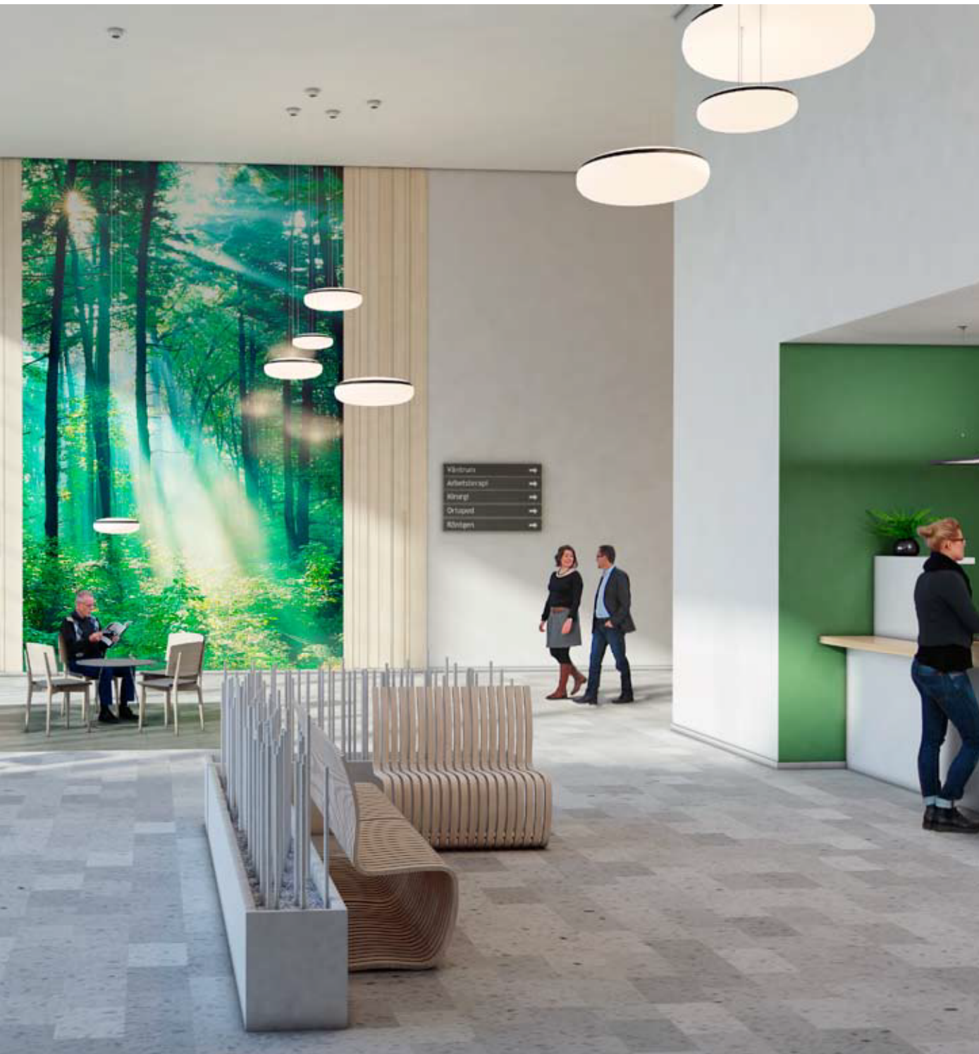
Suspended Tibi luminaires provide the general levels with a direct/indirect distribution, complemented by Appareo over the workstation. The system has been optimised with daylight and presence control to regulate the light levels and reduce the energy consumed.
