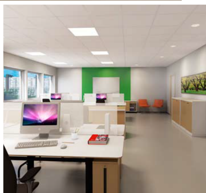
Recessed Multilume Flat, with a large lit surface, provides a well shielded working and general light. The ambient light is enhanced with Pleiad Wallwasher G3. A G5 desk luminaire supplements the fittings within the room to offer individual control of the light.
