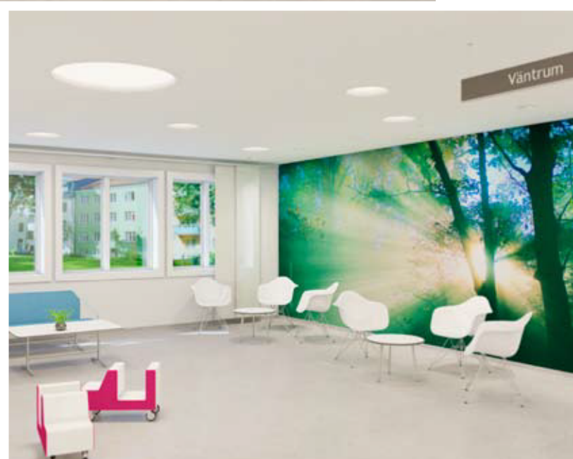
Recessed Pozzo LED acts as a light well or skylight the ceiling, helping to create a feel of natural light where there maybe limits on the real thing. Recessed Pleiad Wallwasher G3 offer more vertical light and accentuate the photo wall.
